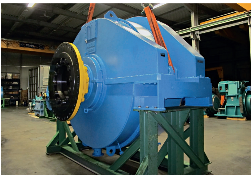
3 Big (38-ton), freshly overhauled planetary stage at Brauer Maschinentechnik AG
